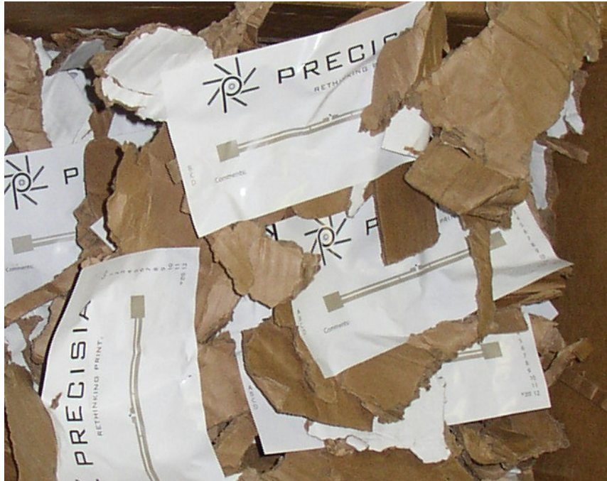
Figure 3.1 Sample of Clippings with RFID Labels Attached
