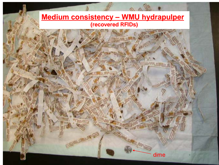
Photo 2 Recovered RFIDs from WMU Hydrapulper
